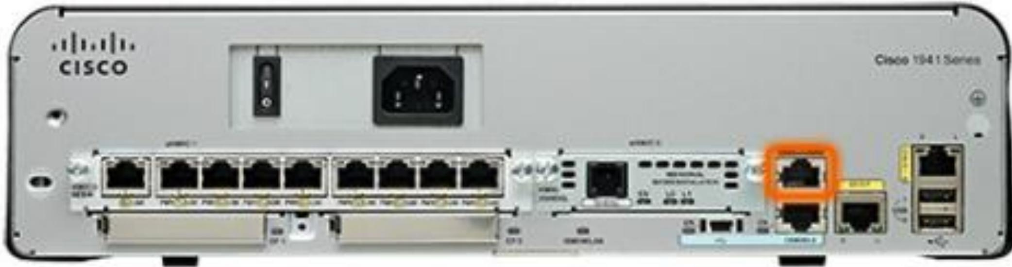
An older way to establish a CLI session remotely is via a telephone dialup connection using a modem connected to the auxiliary (AUX) port of a router
