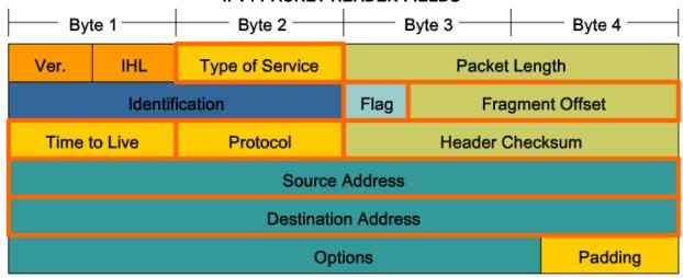
As shown in the figure, an IPv4 protocol defines many different fields in the packet header. These fields contain binary values that the IPv4 services reference as they forward packets across the network.
