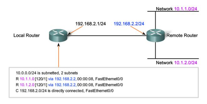
This is the routing table output of Local Router when the "show ip route" is issued.
