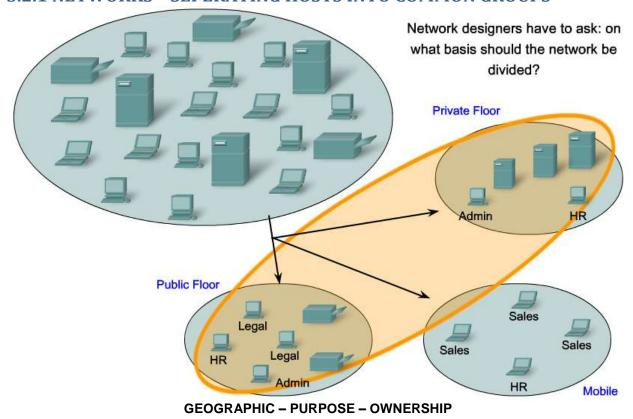
One of the major roles of the Network layer is to provide a mechanism for addressing hosts. As the number of hosts on the network grows, more planning is required to manage and address the network.
