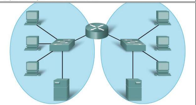
Replacing the middle switch with a router creates 2 IP subnets, hence, 2 distinct broadcast domains. All devices are connected but local broadcasts are contained.
