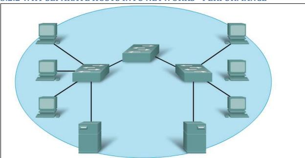
All devices in this network are connected in one broadcast domain when the switch is set to the factory default settings. Since switches forward broadcasts by default, broadcasts are processed by all devices in this network.
