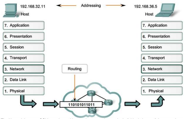
The Network layer, or OSI Layer 3, provides services to exchange the individual pieces of data over the network between identified end devices. To accomplish this end-to-end transport, Layer 3 uses four basic processes:
