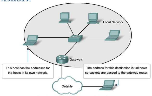
Hosts do not know how to deliver data to devices in a remote network - this is the role of the gateway.
