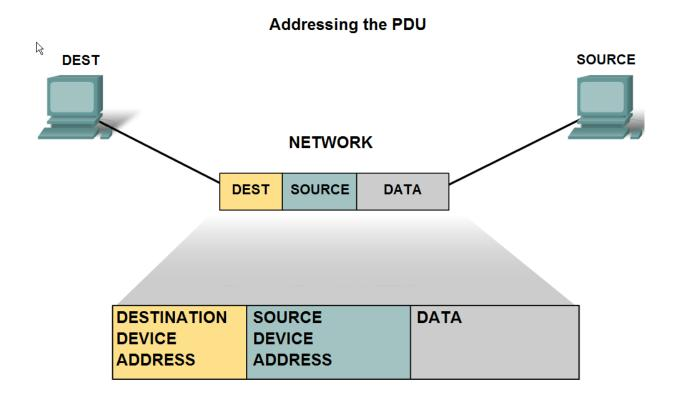
Explain how labels in encapsulation headers are used to manage communication in data networks
