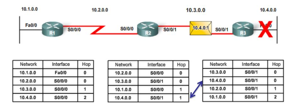
A **routing loop** can occur when two or more routers have routing information that incorrectly indicates that a valid path to an unreachable destination exists.
